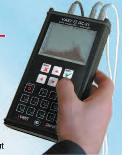
The DC-21® is a fully digital dual channel spectrum analyzer and data collector. It is used for:
