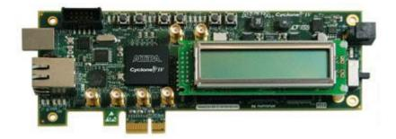
Altera's Cyclone<sup>®</sup> IV GX Transceiver Starter Kit provides a low-cost platform for developing transceiver I/O-based FPGA designs. This kit includes the complete hardware and software for you to:
