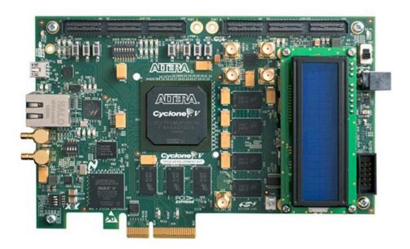
The Altera® Cyclone® V GT FPGA Development Kit can be used to prototype Cyclone V GT FPGA or Cyclone V GX FPGA applications. It offers a quick and simple way to develop low-cost and low-power FPGA system-level designs and achieve rapid results. This kit supports a myriad of functionalities such as:
