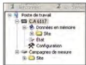
▶ The menu presents the tree structure of the data present in the product and measurement campaigns, clearly identified (customer, location, type of measurements, etc.).
