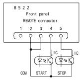
Example of wiring diagram with a logic element
