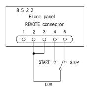
Example of wiring diagram with other controls Fig. 5.4
