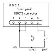
Remote-control box wiring diagram Fig. 5.3
