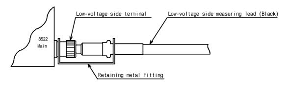
Fix the U-shape part of the retaining metal fitting at the low-voltage terminal of the tester.
