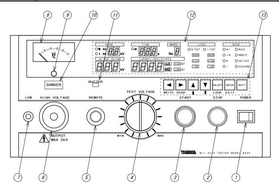
① POWER Power supply switch. Press right to turn ON and left to turn OFF.
