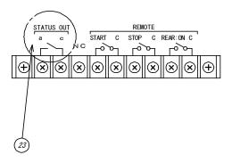
It can be connected to the optional buzzer unit (5858-05) and so on. Plural numbers of output names for status output can be selected (it is OR selection).
