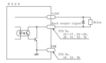
Fig.14.2 Connection example of relay drive
