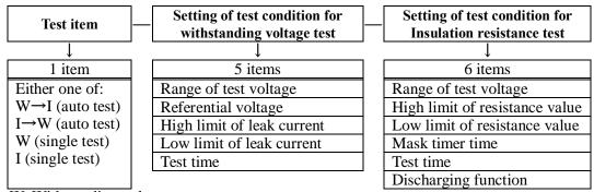
W: Withstanding voltage test I: Insulation resistance test
