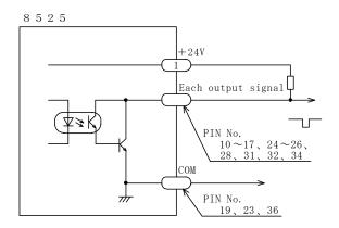
Fig.14.3 Example to obtain a signal level
