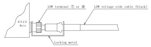
Fasten the U-shape ditch side to the LOW terminal of the tester main unit.
