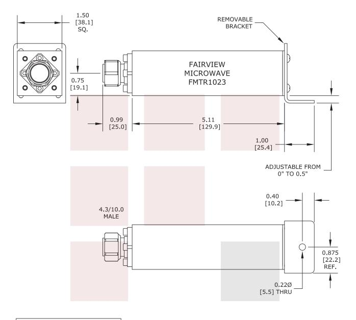
UNLESS OTHERWISE SPECIFIED: DIMENSIONS ARE IN: inches TOLERANCES ARE: [mm] HOLE TOLERANCE: X.XXX ± .003 [±.076] LENGTH TOLERANCE: X.XXX ± .010 [±.254] LENGTH TOLERANCE: X.XX ± .030 [±.762]
