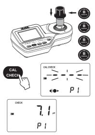
The reading should be within specifications as reported in the CAL CHECK<sup>TM</sup> Standard Certificate. If the value is found out of the specifications, please check that the cuvettes are free of fingerprints, oil or dirt and repeat validation. If results are still found out of specifications, then recalibrate the instrument.
