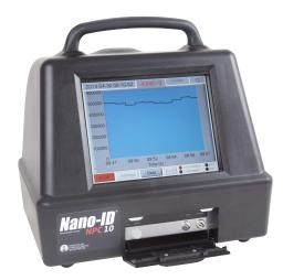
The Nano-ID NPC10 is the first Condensation Particle Counterspecifically developed for ultra-clean manufacturing environments. This instrument combines 10 nm sensitivity with high sample flowrate and the lowest zero count specification on the market.
