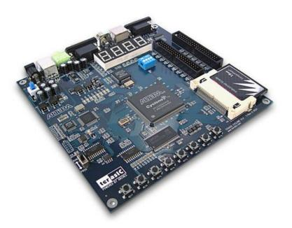
The TREX C1 Development Kit provides a complete, high-quality, multimedia platform featuring Altera Cyclone (EP1C6Q248C8) FPGA device. With the built-in USB blaster circuits, the TR1 development board has many multimedia features for users to develop advanced video, audio, memory and storage applications using the most popular components in consumer electronic products such as DVD and VCD players.
