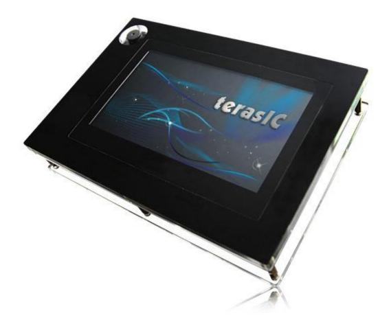
The Video and Embedded Evaluation Kit - Multi-Touch for SoCKit Upgrade Kit( VEEK-MT-SoCKit Upgrade Kit ) offers customers who already own a SoCKit board a brand new integrated platform to develop various embedded applications. We provide simple and straightforward installation guidelines for users to assemble their already owned SoCKit with this upgrade kit.
