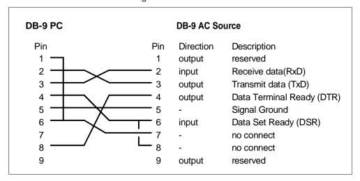
Figure 8-3: RS232C Interface Cable Wiring Diagram
