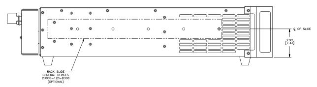
Figure 2-2: Rack Mount Slides (-RMS option) position
