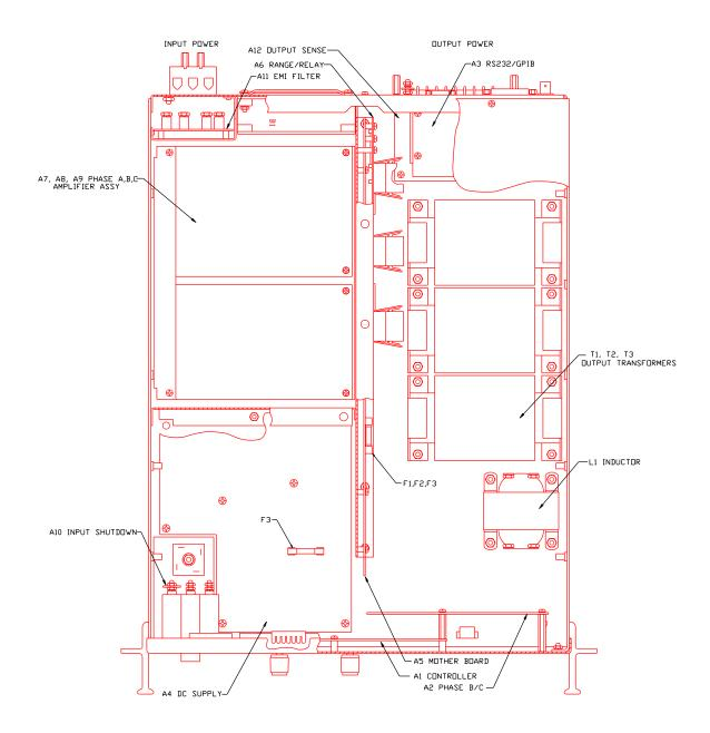
Figure 7-1: Assembly Location
