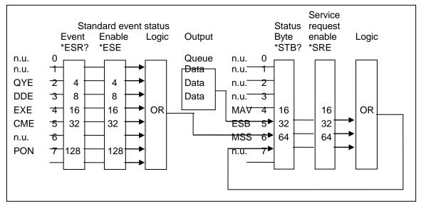
Figure 12-1: AC Source Status System Model
