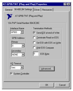
Figure 8-7: NI AT-GPIB/TNT Settings
