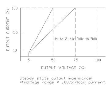
Figure 2-1: Available RMS Current as function of Output Voltage and Frequency.
