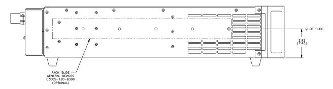
Figure 3-5: Rack Mount Slides (-RMS option) position
