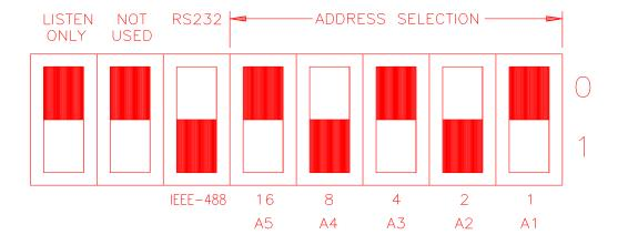
Figure 8-2: GPIB Address Selection Switch
