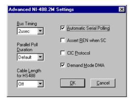
Figure 8-8: NI AT-GPIB/TNT Advanced Settings Dialog
