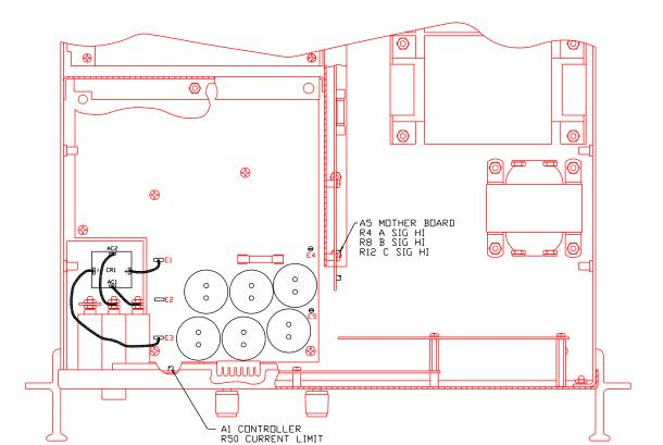
Figure 3-4: Internal Jumper Location, Input Line Voltage 208/230
