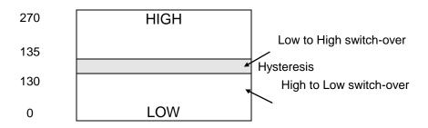
Figure 4-2: Voltage Auto Range Switch Over Points
