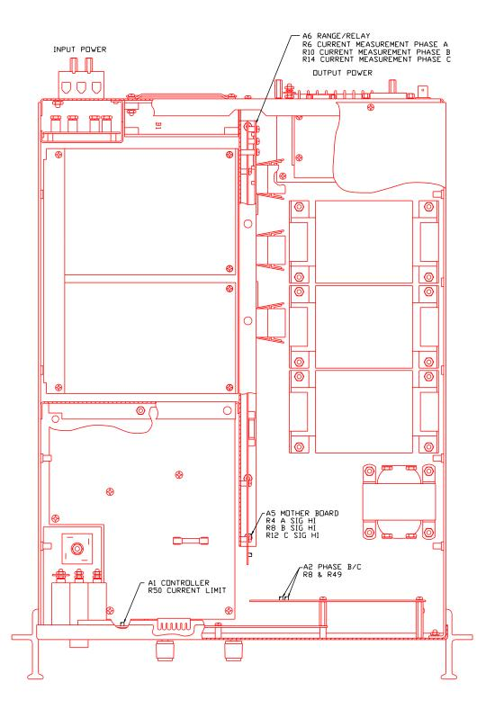
Figure 6-3: Internal Adjustments
