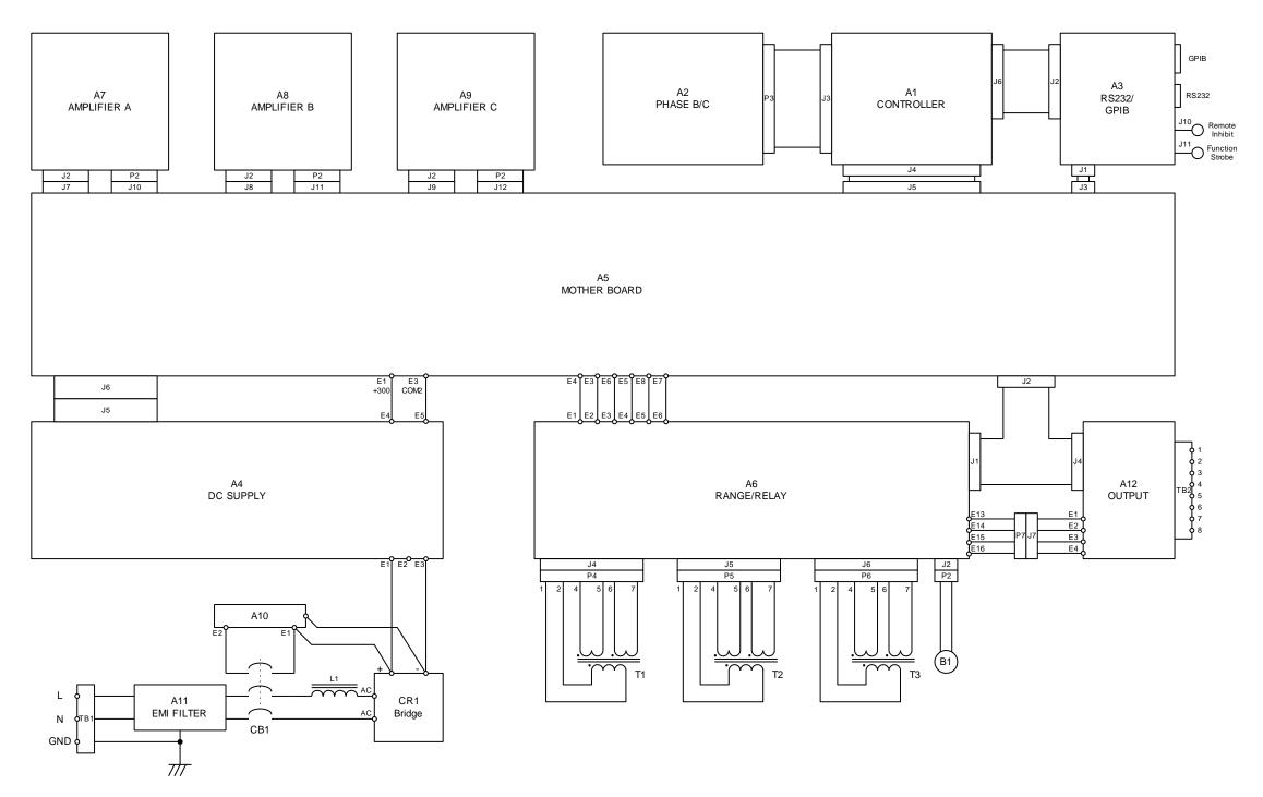
Figure 5-1: AC Power System Block Diagram
