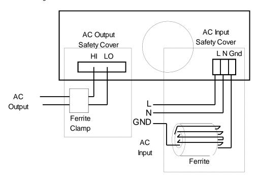
Figure 3-6: Input and Output Wiring
