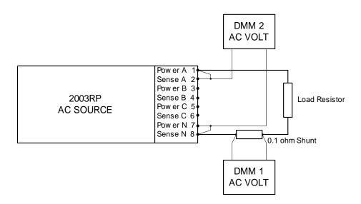
Figure 6-2: Test Equipment Hook-up for Current and Power Measurement Calibration
