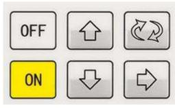
ON: OFF: Arrow keys up / down / right: Shift key: switch on device switch off device select decimal place and set sound velocity switch between normal measurement mode, calibration mode and sound velocity selection
