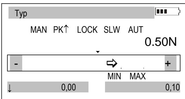
Changing actual force value indication into peak value measurement is done by pressing *PEAK* key. Indication stabilization sign changes into *LOCK* sign and force meter changes mode into peak value for force in both directions. Pressing again *PEAK* key changes mode into one-direction peak value: first for pressure force (*PK↑*) and after another *PEAK* pressing for pulling (*PK↓*), zeroing is done by *→0←* key.
