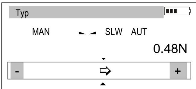
The force measurement is continuous. Display continuously indicates actual force value measured by meter. Force direction is signalized by an arrow in lower part of screen and a sign + (pressing force) or - (pulling force). Saving actual force indication to memory is done by pressing *MEM* key.
