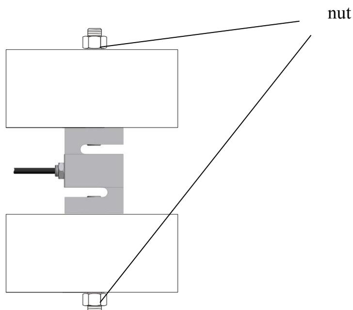
Screw connection should be realized using screws with proper thread that ensure connection endurance not less than 150% of force gauge measuring (150% Max).
