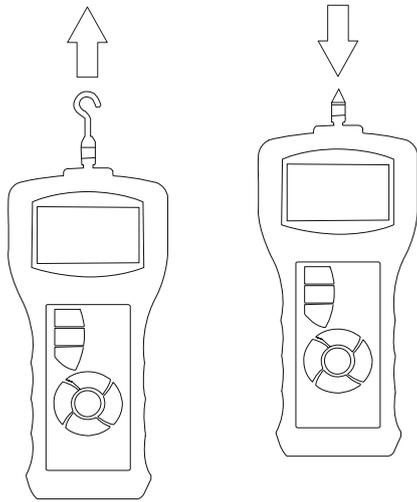
Before starting the measurement, choose a suitable measurement tip, screw it to the gauge plunger and reset the gauge in the operating position, e.g. horizontal position (laying the gauge on a table).
