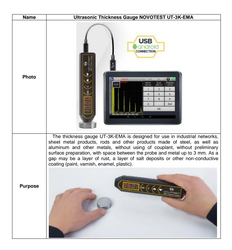
The readings of the device are slightly affected by skew, in contrast to traditional thickness gauges with piezoelectric transducers, which require fixation of the probe in a certain position. The thickness gauge UT-3K-EMA uses a special data processing algorithm that allows the thickness to be measured correctly in the presence of disturbing factors such as metal anisotropy, the presence of several reflectors, and the presence of external interference.
