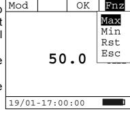
By pressing key **F3** (**OK**), the selected item is confirmed. To the side, an example of measurement with active Max function. The display shows the active function.
