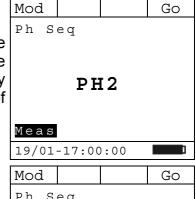
7. If there is concordance between the two phases, to which the test lead has been connected, the instrument displays the screen here to the side. Otherwise, it displays "123" or "132".
