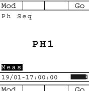
4. Once phase L1 acquisition is complete, the displays shows the screen here to the side. Disconnect the test lead from phase L1 cable.
