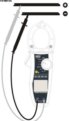
Fig. 5: DC voltage measurement
