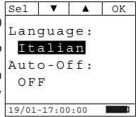
• Auto-Off: the auto power off of the clamp may be set to ON or OFF. If set to ON, the clamp will switch off after 5 minutes after it is last used.
