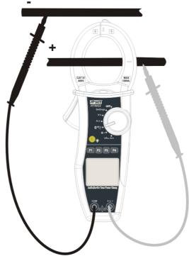
Fig. 11: DC power measurement
