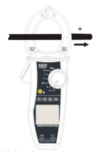
Fig. 14: inrush current measurement
