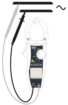
Fig. 6: AC+DC voltage measurement
