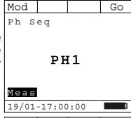
4. Once phase L1 acquisition is complete, the displays shows the screen here to the side. Disconnect the test lead from phase L1 cable.
