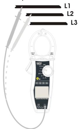
Fig. 7: verification of phase sequence
