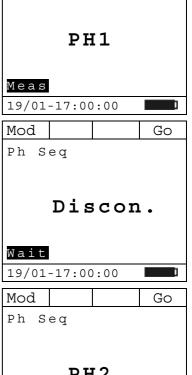
5. The instrument shows the screen here to the side, and waits for the detection of the second sequence of phase L1. Connect the test lead to phase L1 of the second sequence.
