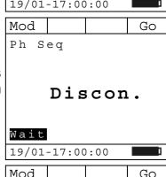
The instrument shows the screen here to the side, and waits for the detection of phase L2. Connect the test lead to phase L2 cable.
