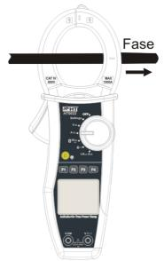
Fig. 10: AC+DC current measurement
