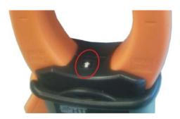
The photo in Fig. 4: current direction arrow shows an arrow which indicates the conventional direction of current.
