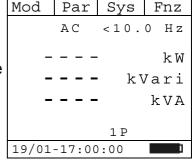
Press key **F1** (**Mod**) to open the drop-down menu shown on the screen to the side. At each subsequent pressure of key **F1**, the cursor will scroll through the available items, as follows:
