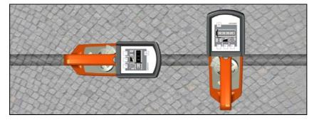
Fig. 12: Alignment of the receiver RX5000
