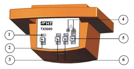
Fig. 3: Front panel of transmitter TX5000
