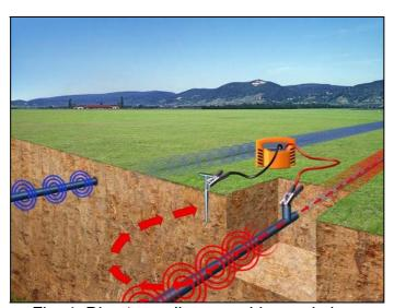
Fig. 4: Direct coupling on cables and pipes
