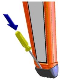
Fig. 14: Replacement of the floor cap
