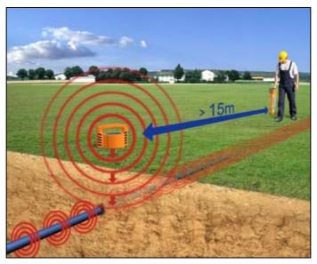
Fig. 7:Inductive signal coupling
