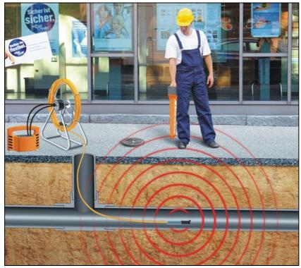
Fig. 9: Signal coupling in non-metallic pipes
