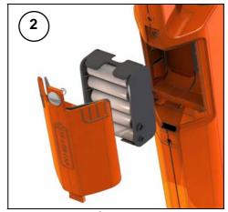
Fig. 15: Replacement internal batteries of RX5000
