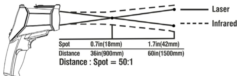
Fig. 27: Diameter of surface S with reference to the distance D from the object (in mm)
