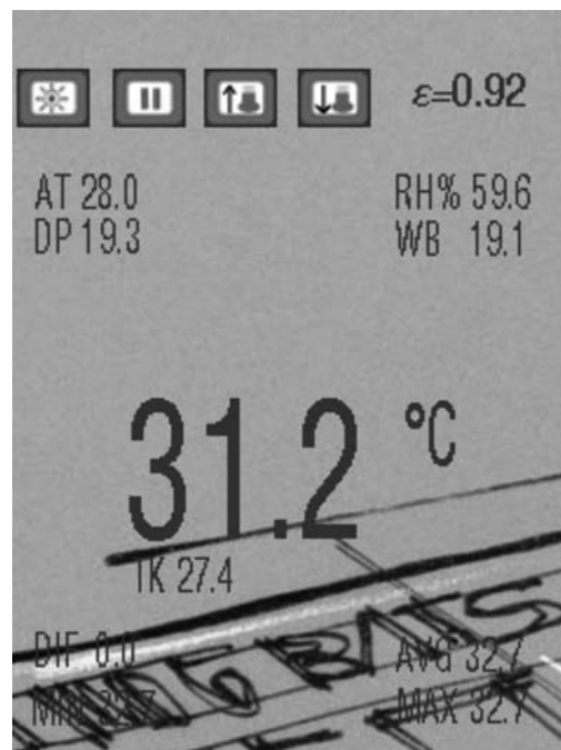
Fig. 26: IR temperature measurement with in-built photo camera
