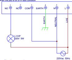
Example three: Signal lamp connection
