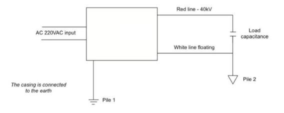
Wiring description: The grounding bolt of the rear panel of the product is grounded by the pile 1. The black terminal of the rear panel is connected to the floating white line, and the capacitor is negative, that is, the ground pile 2 in the above figure.
