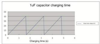
Continuous charge and discharge curve
