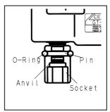
If it is not securely attached, the socket or bit may detach and fly off. Do not attach the socket or bit when the tool is idling.
