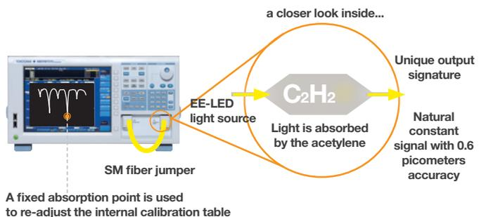
The built-in reference source for wavelength calibration, available for AQ6370D, AQ6374, AQ6375B and AQ6376.
