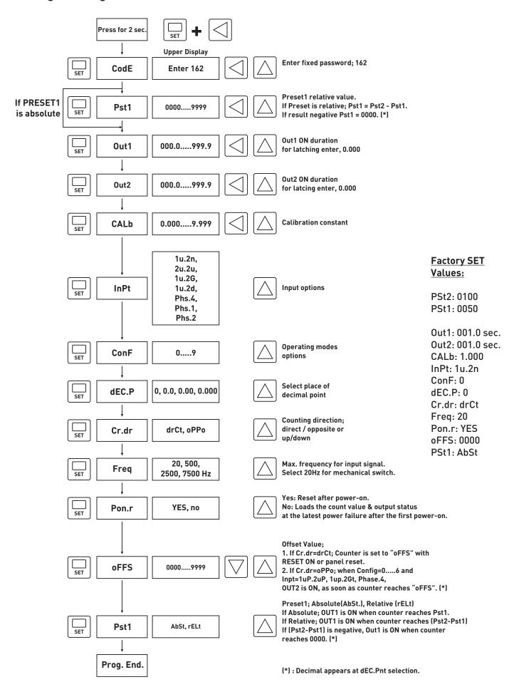
Note: If no entry is done for 20 sec. during programming, current enteries are accepted and saved to EEPROM memory.
