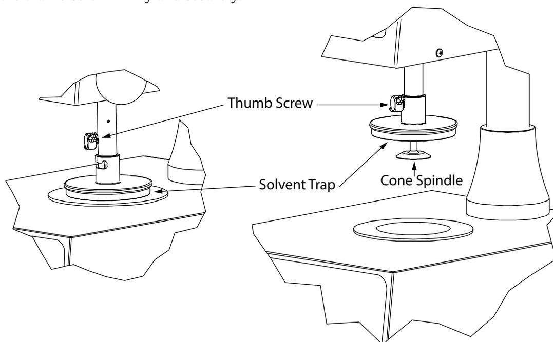
**Figure II-3: Cone Attachment**
