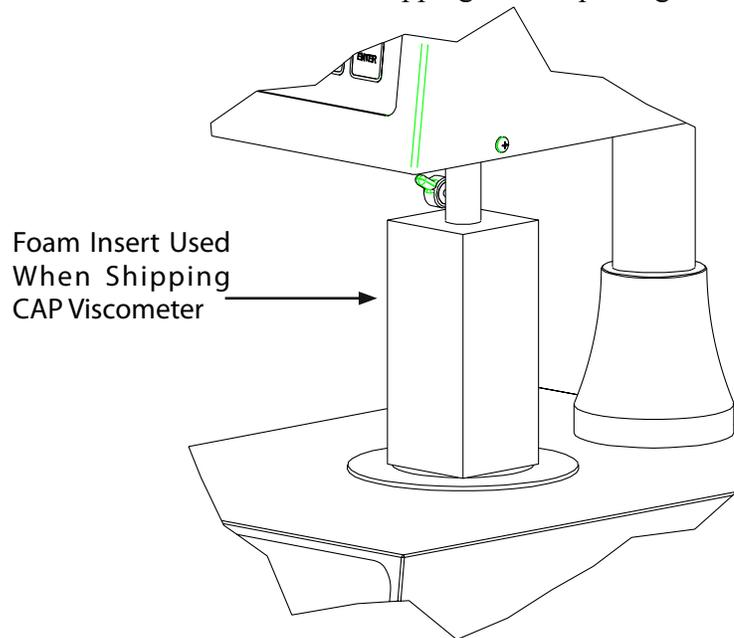
**Figure I-2: Detail of Foam Insert**
