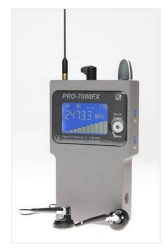
bug detectors. Such devices include GPS Trackers and GSM (Mobile phone) based devices where a 'Burst' signal or SMS (Text Messages) are sent momentarily. The PRO7000FX will alert you if a device has transmitted within the vicinity even for just a fraction of a second.
